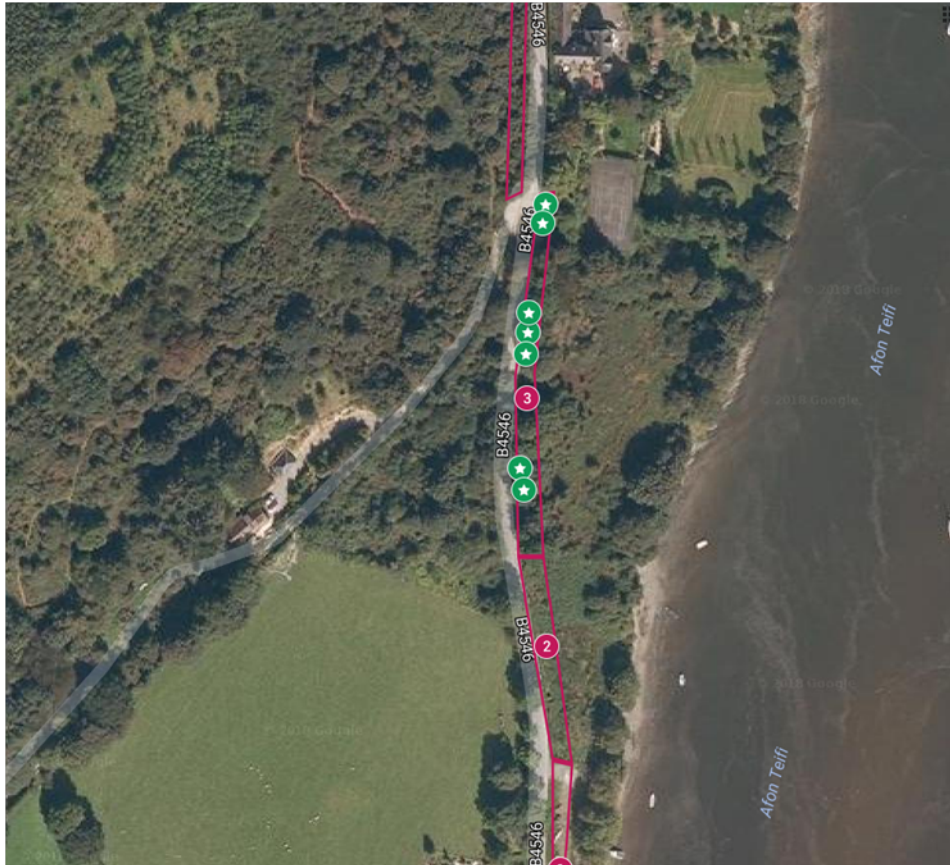
Figure 8. Green stars represent locations of mature trees (>30cm trunk diameter) in Area 2 which may have to be felled due to path construction.
